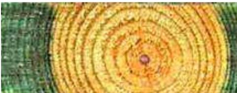
Example of excessive unpenetrated heartwood in CCA-treated pine sleeper, revealed after docking an end and using a colour indicator.
