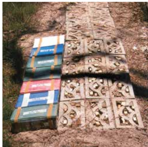
Figure 4. Field exposure to subterranean termites using a brick-assembly technique.
