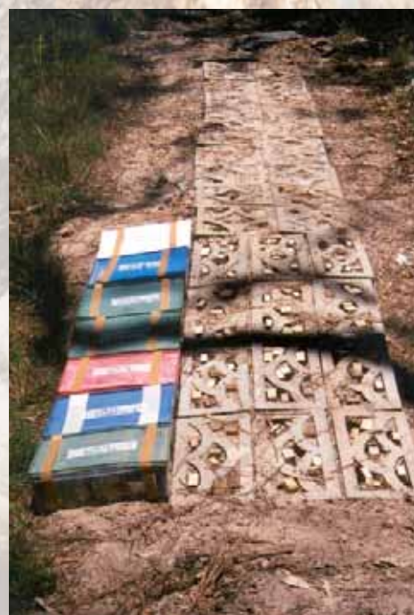
Figure 3. Field exposure to subterranean termites using a brick-assembly technique.
